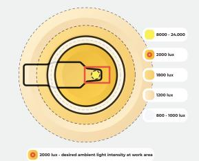
This diagram illustrates the optimal light distribution in a dental treatment room, aiming for 1500-2000 lux around the oral cavity.
