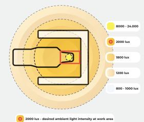
This diagram illustrates the optimal light distribution in a dental treatment room, aiming for 1500-2000 lux around the oral cavity.
