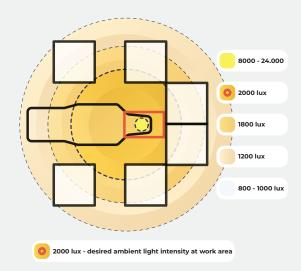
This diagram illustrates the optimal light distribution in a dental treatment room, aiming for 1500-2000 lux around the oral cavity.
